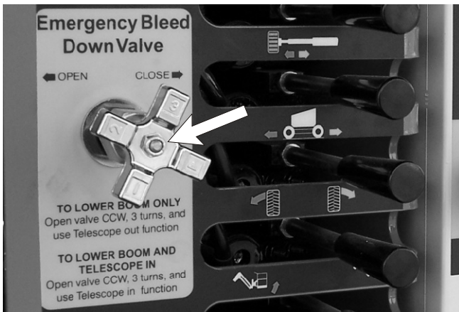
Figure 3.4—Emergency Lowering Knob
